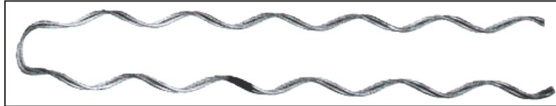
The service ends is conceived to attach the service cable to its end point and is designed for bare neutral-messenger of self-supporting cable used in making service drops. This product is produced in galvanized steel class A, grade 180 (CSA-G12 / ASTM-A475) standard and class **B** upon request.
